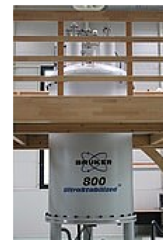
Magnet of 18.8 T from Chevreul Institute (Villeneuve d'Ascq) 1 H, 13 C and 31 P resonate at 800, 13, 201.2 and 323.9 MHz respectively
